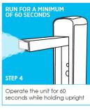
Flyp Tip: If a user reports a decreased flow output or lengthening treatment times, its usually an indication of the holes becoming clogged. Distilled white vinegar is an excellent organic solvent to provide a deep cleaning. Simply fill the medication reservoir with a bit of the vinegar and power the unit on to run for one cycle. We recommend doing so in a well ventilated area.
